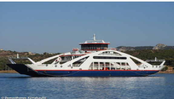
Type: RO-RO PAX | L x B : 74,9 x 15,7 | GT : 968 | Built: 2018 Capacity: 494 PAX | 86 vehicles | Flag: Greek
