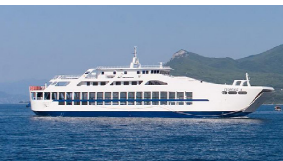
Type: RO-RO PAX | L x B : 72,2 x 16,00 | GT : 1147 | Built: 2018 Capacity: 500 PAX | 100 vehicles | Flag: Greek
