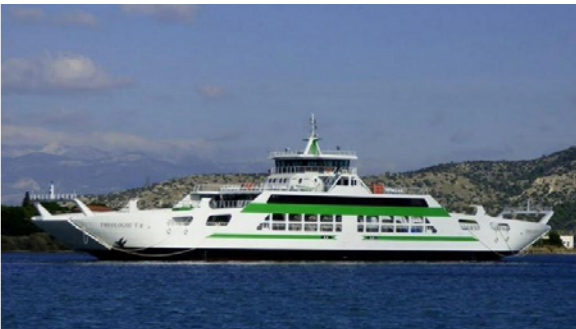
Type: RO-RO PAX | L x B : 93,12 x 17,56 | GT : 1367 | Built: 2018 Capacity: 450 PAX | 126 vehicles | Flag: Greek
