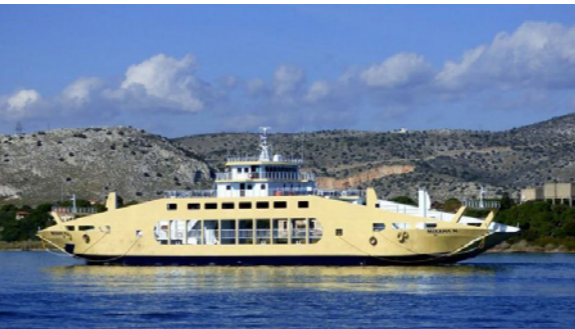
Type: RO-RO PAX | L x B : 78,6 x 16,5 | GT : 1045 | Built: 2018 Capacity: 308 PAX | 87 vehicles | Flag: Greek
