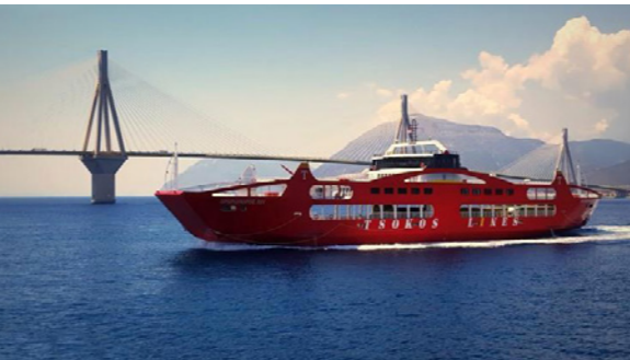
Type: RO-RO PAX | L x B : 99,65 x 18,00 | GT : 1857 | Built: 2018 Capacity: 900 PAX | 148 vehicles | Flag: Greek
