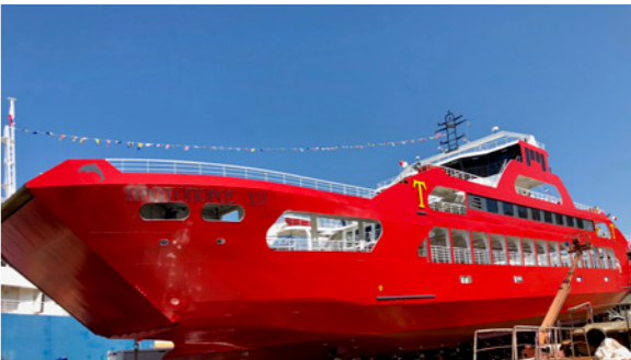
Type: RO-RO PAX | L x B : 91 x 17,56 | GT : 1482 | Built: 2018 Capacity: 800 PAX | Flag: Greek
